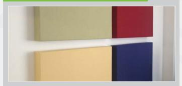
The Hush Absorber 50 is a Class A Absorber that works using a specially formulated 50mm thick acoustic foam and is hand finished with interior fabric that is applied to the face, edges and back return.
