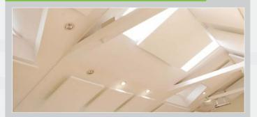
The Hush Absorber 50A is a Class A Absorber which consists of fabric wrapped 50mm thick acoustic foam, with built in support frames to allow for bracket fixing to provide an air void behind the absorber for enhanced acoustic performance.
