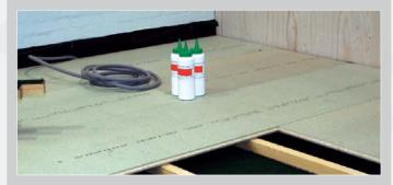
Hush Batten 55 has been designed as a resilient composite batten used to enable the construction of a service void, whilst reducing impact sound transmission and providing long lasting support for floating timber or chipboard floors.
