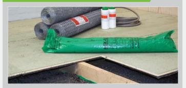
Hush Fill 60 Heavy Pugging is a granular mineral filler specifically designed to meet the required density of 80kgs/m² at the 60mm regulation depth specified within UK Building Regulations for sound insulation between timber floor joists.
